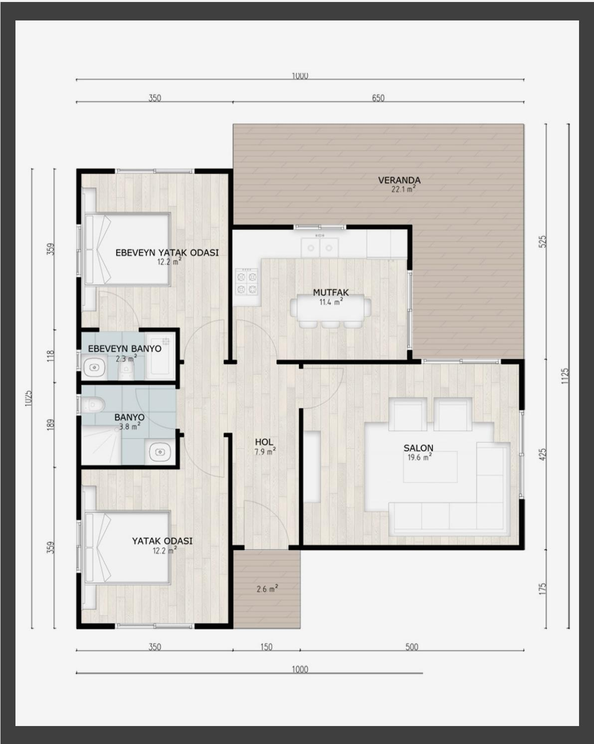
The SM-1100 project covers a total area of 100 m<sup>2</sup>, offering a 2+1 room layout with a closed kitchen. Its L-shaped veranda connects to the kitchen from both directions and directly to the living room, providing seamless indoor-to-outdoor transitions. The master bedroom includes an en-suite bathroom, and the expansive windows in all rooms, including the living room, create a bright and airy environment.
