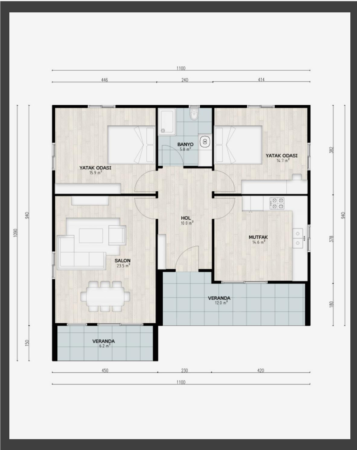
The SM-1110 project is a 110 m<sup>2</sup> light steel construction home with a 2+1 room layout and a closed kitchen. It creates a spacious and airy environment with its 4,5-meter-high ceilings. The design incorporates custom windows that allow ample sunlight and provide an immersive connection to nature.
