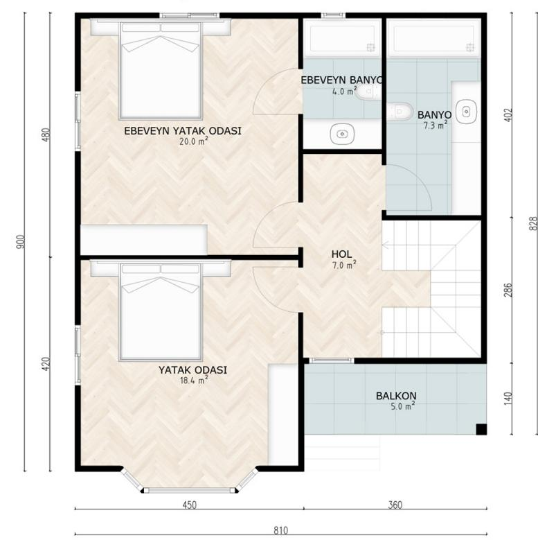
The ST-2144 project is a luxurious 144 m<sup>2</sup> two-story light steel construction home with a 3+1 room layout. It features a stunning fully glass bay window design and a four-gable roof system, providing both visual and functional elegance. Large windows ensure spacious and bright interiors.
