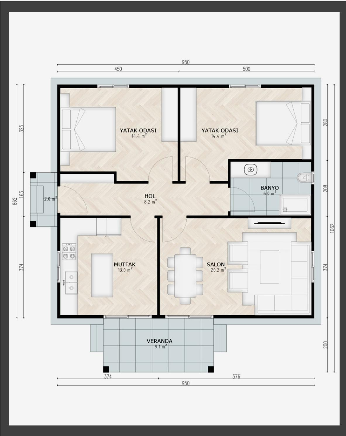
The SM-1093 project is a 93 m<sup>2</sup> light steel construction home with a 2+1 room layout and a closed kitchen. Its four-gable roof showcases the durability and security of light steel construction. The design successfully combines modern aesthetics with classical architectural lines for an elegant and visually appealing structure.
