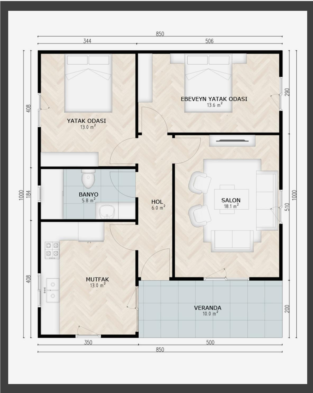
The SM-1085 project is an 85 m<sup>2</sup> light steel construction home with a 2+1 room layout and a closed kitchen. Its veranda features fiber cement cladding that improves thermal and sound insulation while adding the natural aesthetic of wood. The high-pitched gable roof is specifically designed to withstand strong winds and heavy snow loads, making it particularly suitable for colder climates.
